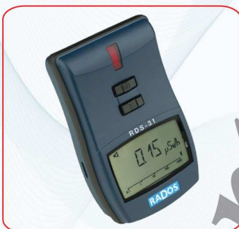
Dose rate : 0.01 \mu Sv/h-0.1mSv/h or 1 \mu rem-10rem/h Dose : 0-0.1 \mu Sv/h- 10Sv or 1 \mu rem- 1000rem Energy : 48keV-3MeV
